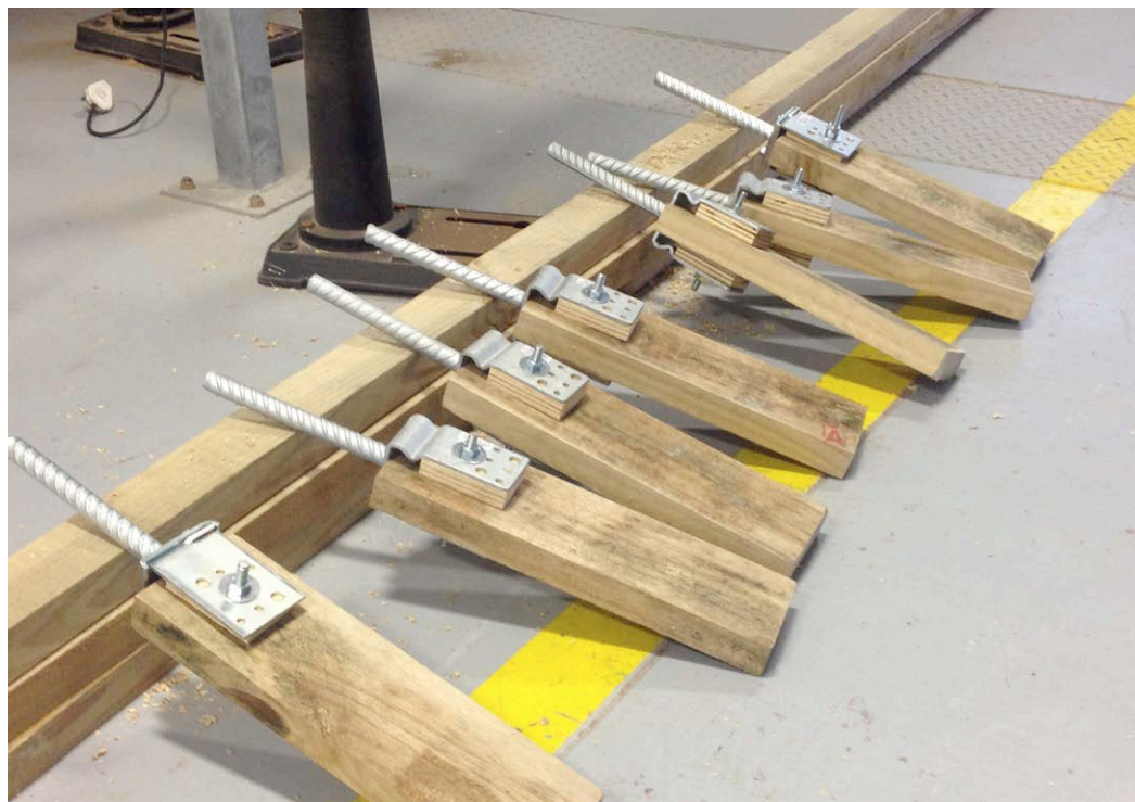
Base Fittings of Triple-Columns
