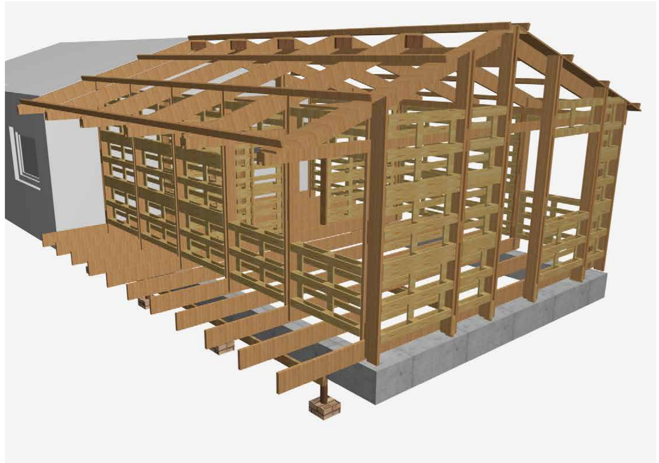
Structure consisting of recycled pallets and structural timber members
